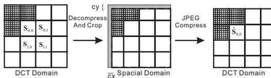
Fig. 2. Generation of an SD-JPEG image.
