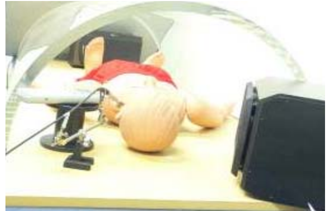
Fig.2. Block diagram and photograph of the laboratory experimental setup. Primary loudspeaker is placed on the one end of the bore. Reference microphone is placed close to the primary speaker. Canceling loudspeaker is placed on the other end of the bore, close to the head of the manikin. Error microphone is placed close to the ear of the manikin. SPL meter measures the error sound level.
