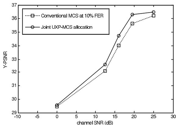
**Fig. 2.** Comparison of PSNR performance of the Football sequence between the proposed joint UXP-MCS allocation and the conventional MCS allocation for different channel SNR regions. The points are plotted in the middle of each SNR region specified in Table 1.
