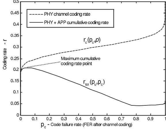
**Fig. 1.** Example of the optimal operating point  $(p_c, r_{\text{total}})$  that maximizes the cumulative throughput  $r_{\text{total}}$  while satisfying the UXP error requirement  $p_u$ . The dotted curve shows the channel coding rate  $r_c$  as a function of the FER  $p_c$ . The solid line shows the cumulative coding rate  $r_{\text{total}}(p_c, p_u, \rho)$  as a function of  $p_c$  for a target UXP rate  $p_u$  and an uncoded channel rate  $\rho$ .
