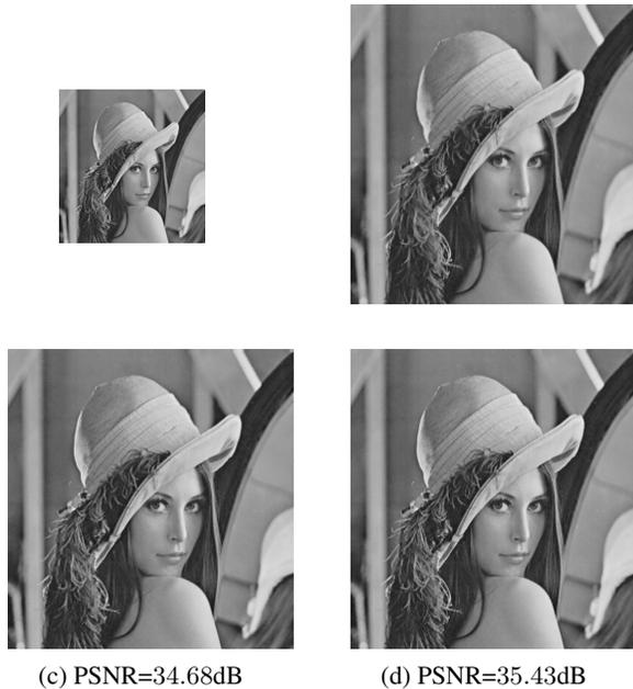
**Fig. 5.** The image Lena is interpolated from the size  $256 \times 256$  to the size  $512 \times 512$  pixels using the three methods: simple interpolation with the Haar filter, wavelet-based and interpolation based on directionlets. (a) The LR image. (b) Interpolation using the Haar scaling function (PSNR=31.56dB). (c) Locally adaptive wavelet-based interpolation [7] (PSNR=34.68dB). (d) Interpolation based on directionlets (PSNR=35.43dB).
