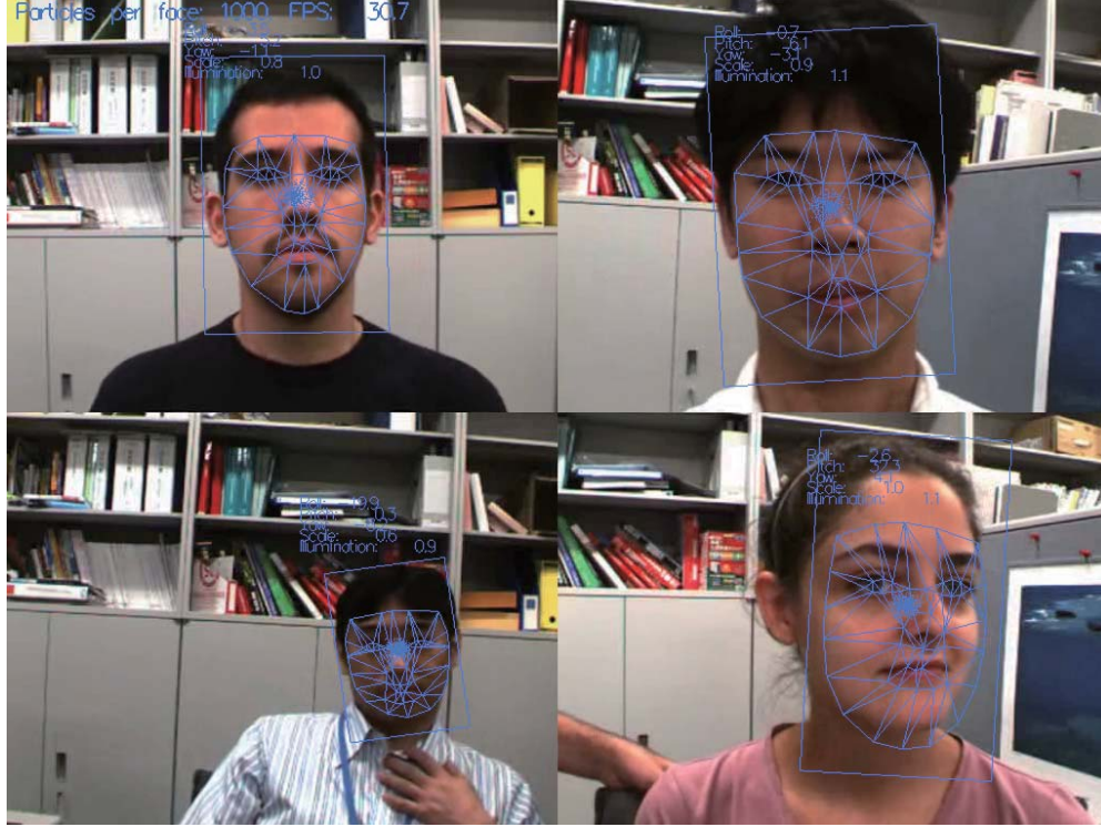
Fig. 1. Results of the simultaneous tracking of four faces. The frame sequence is taken from a synthetic 1024x768 video, the sparse templates are composed of approximately 230 feature points, and each one is tracked using 1000 particles.
