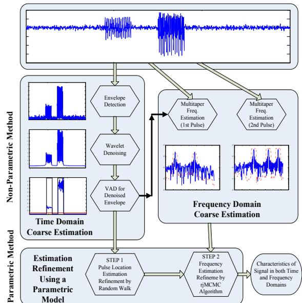
Fig. 1. Procedure for the whole estimation system
