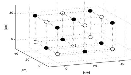
**Fig. 2.** Geometry of microphone positions for filter design (white) and validation (black).
