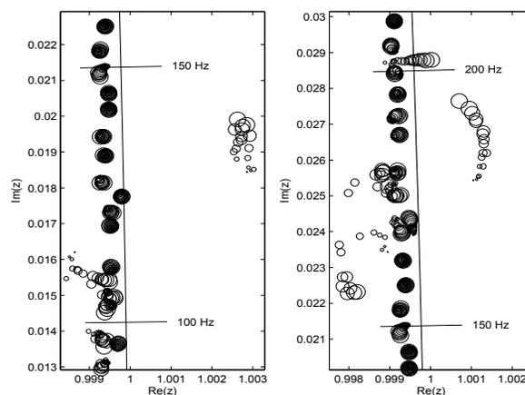
**Fig. 1.** Zeros of 18 transfer functions, acquired from microphone positions along a line. Zeros are represented by circles, where different radii are used to distinguish individual microphone positions. The smallest and largest radii represent the start and stop positions, respectively. The two diagrams represent zoomed segments of the complex plane near the unit circle, at 100 – 150 Hz (left) and 150 – 200 Hz (right).
