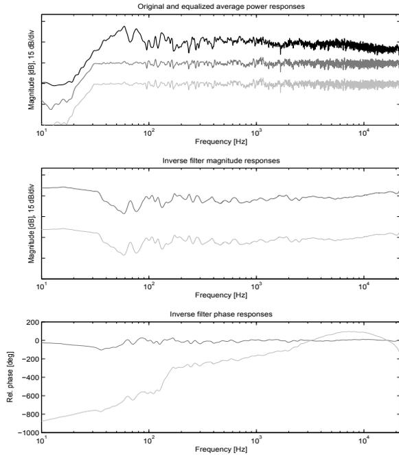
**Fig. 3.** Original and equalized average power responses, measured in the room (top). Magnitude and phase responses (middle and bottom, respectively) of inverse filters. Dark and light grey curves represent minimum phase and mixed phase filters, respectively.
