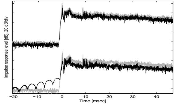
**Fig. 4.** Impulse response maximum level envelopes  $L(k)$  of minimum phase equalization (top) and proposed method (bottom). The grey lines represent the unequalized responses.
