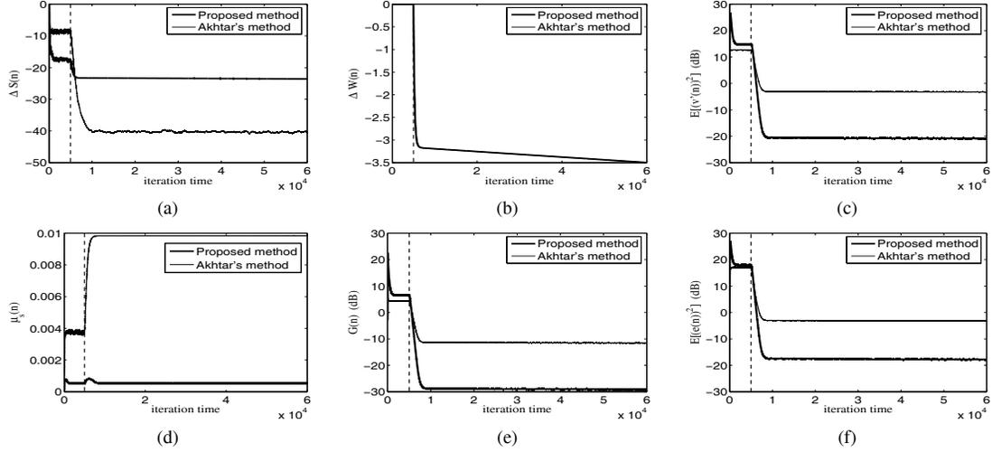
**Fig. 2.** Performance comparison of the ANC system equipped with the auxiliary noise power scheduling of (13) (proposed method), and the ANC system equipped with the auxiliary noise power scheduling of (7) (Akhtar's method).
