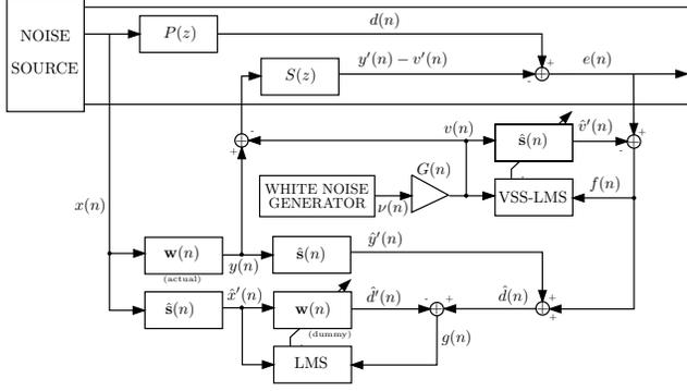
**Fig. 1.** The ANC system with secondary path modeling of Akhtar, Abe, and Kawamata.
