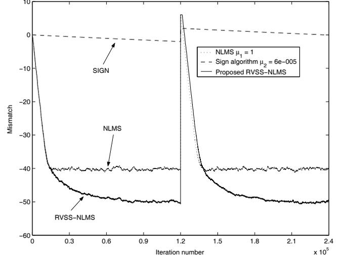
**Fig. 2:** Mismatch (in dB). AR1(0.8) input. No impulsive noise. SBNR=40 dB. The curves are the result of a single realization of the algorithms.
