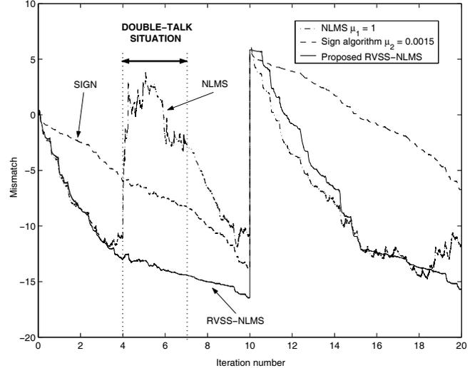
Fig. 4: Mismatch (in dB) for speech input. SBNR=20 dB. STNR=0 dB.
