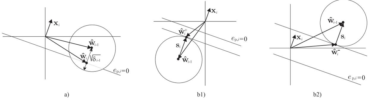
**Fig. 1:** a) In this case, an infinite number of solutions exists (represented by the dotted line). Out of those solutions, we choose that which provides the lowest energy in the update. b1) and b2) Two updates,  $\hat{\mathbf{w}}_i^+$  and  $\hat{\mathbf{w}}_i^-$ , are possible depending on the relative position between the hyperplane and the hypersphere.
