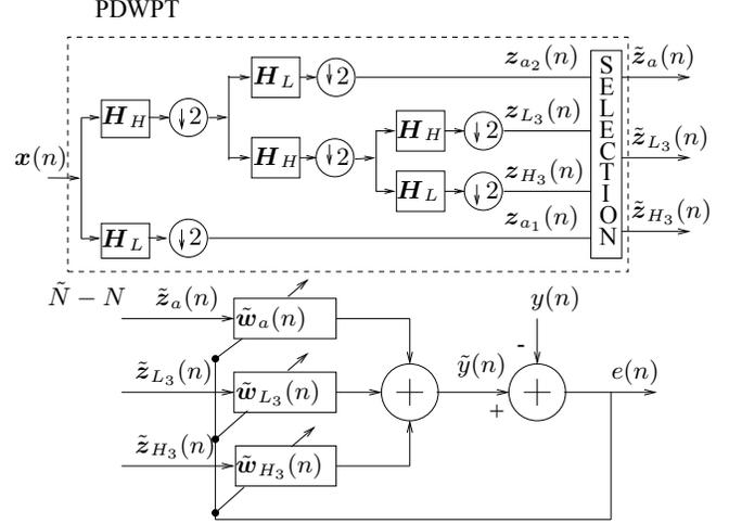
Fig. 1. Block diagram with 3 levels.
