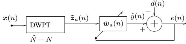
Fig. 4. Block diagram for the 2nd phase of WPB.
