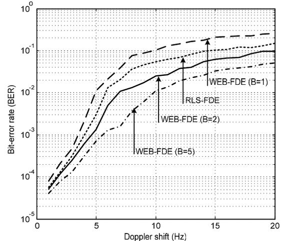
Fig. 3. BER performances according to Doppler shift.
