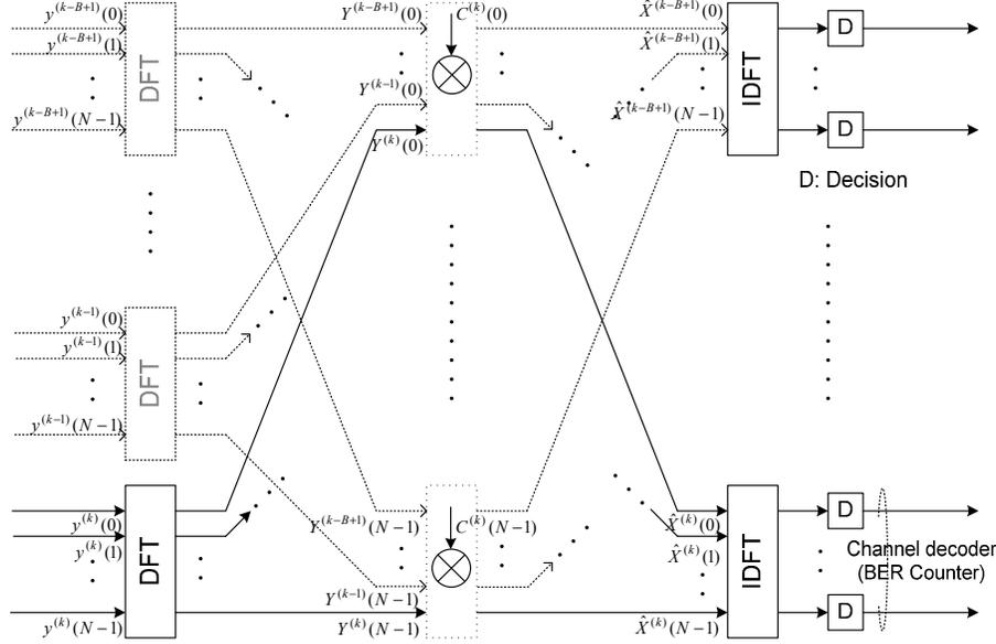
Fig. 1. The conceptual structure of the element-wise block adaptive frequency-domain equalization.
