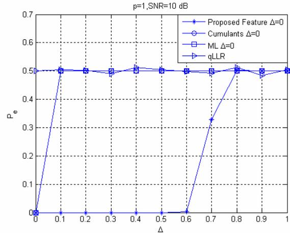
Figure 4: Probability of misclassification ( $P_e$ ) for 2000 PSK2 and PSK4 signals. 1000 realizations for each modulation. Acronyms are the same as for Figure 3.  $p=1$  and  $N=500$ .
