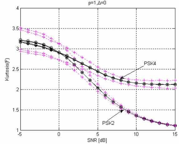
Figure 2: Kurtosis of  $F(k)$  for 6000 PSK2 and PSK4 signals. 3000 realizations for each modulation. Solid lines with \* are the mean and the dotted lines are the mean+standard deviation and the mean-standard deviation, all obtained by simulation. Solid lines with o are the calculated theoretical curves.  $\Delta = 0$  and  $p=1$ .
