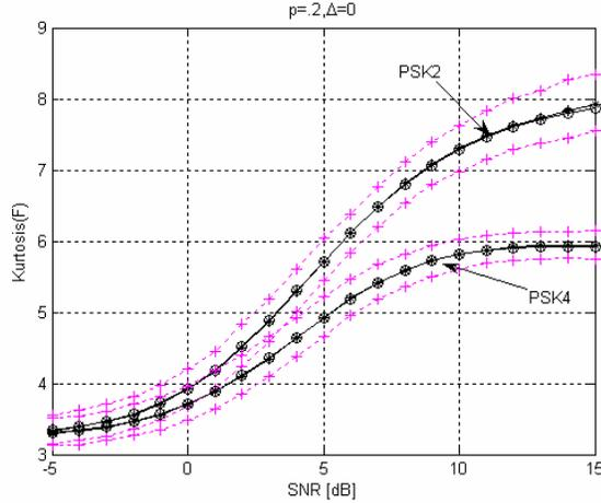
Figure 1: Kurtosis of  $F(k)$  for 6000 PSK2 and PSK4 signals. 3000 realizations for each modulation. Solid lines with \* are the mean and the dotted lines are the mean+standard deviation and the mean-standard deviation, all obtained by simulation. Solid lines with o are the calculated theoretical curves.  $\Delta = 0$  and  $p=2$ .
