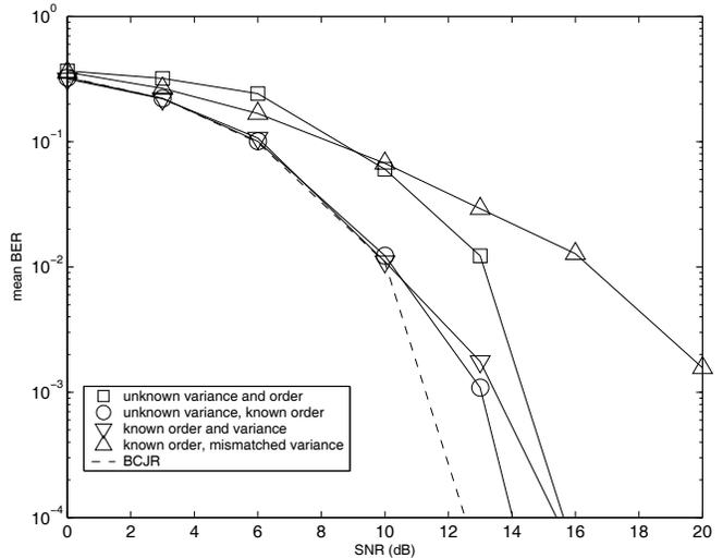
**Fig. 1.** Performance of blind equalization algorithms as a function of the signal-to-noise ratio (SNR) compared to the optimal (BCJR) algorithm. The “unknown variance” curves refer to the proposed method, while the other results employ the method described in [1].
