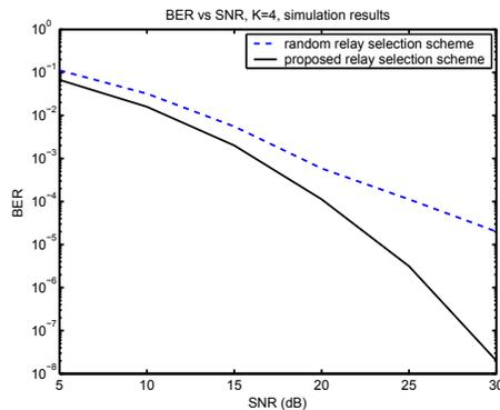
Fig. 2. BER vs SNR for K=4: Simulation results for the proposed relay selection scheme and that of the original ALLIANCES.
