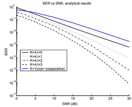
Fig. 1. BER vs SNR, variable  $K$  and  $l$ : analytical results.
