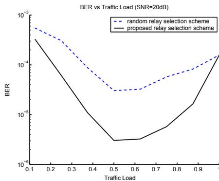
Fig. 3. Simulation results: BER vs traffic Load for  $J=16$ ,  $SNR=20$  dB, and ML decoding.
