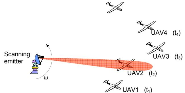
**Fig. 1.** Scan-based geolocation where the  $t_k$  correspond to time instants the emitter beam is intercepted by UAV receivers.
