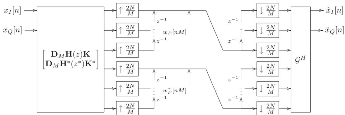
Fig. 5. A general oversampled WL OQPSK communication model.
