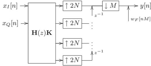
Fig. 2. The PCM form for the overall channel matrix.
