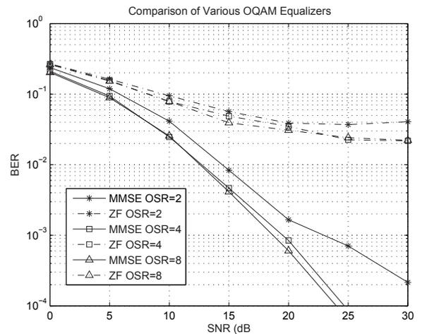
Fig. 4. BER curves for various OQPSK equalizers in Ex. 2
