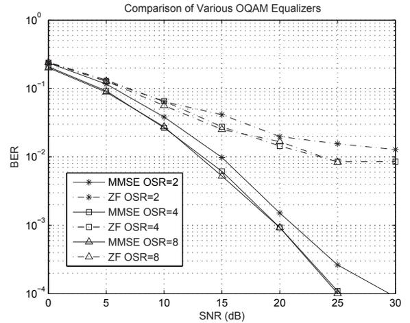
Fig. 3. BER curves for various OQPSK equalizers in Ex. 1
