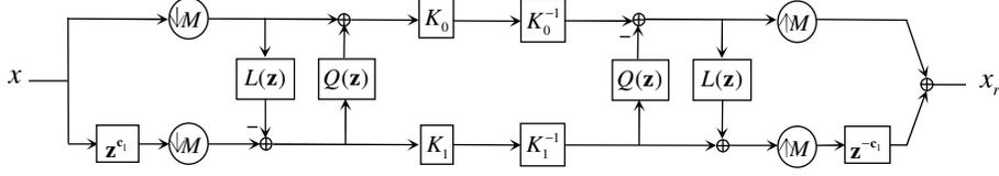
Fig. 3. A two-channel multidimensional filter bank using a two-step lifting scheme.
