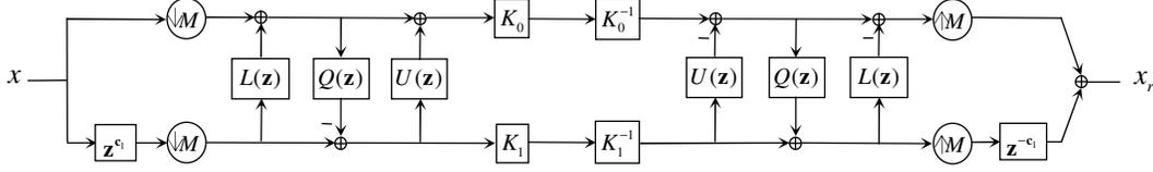
Fig. 4. A two-channel multidimensional filter bank using a three-step lifting scheme.
