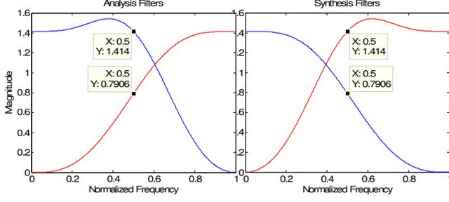
Fig. 2. The frequency response of the analysis filters in Example 1.
