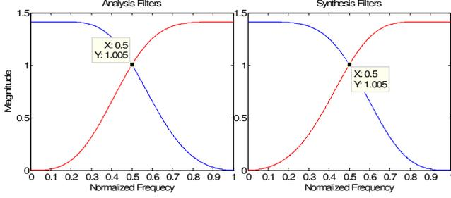
Fig. 5. The frequency responses of the filters in Example 3.
