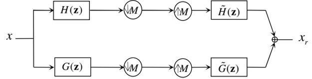
Fig. 1. A two-channel multidimensional filter bank.
