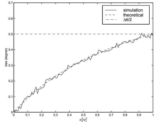
Fig. 3. Comparison of the bias of the DOA estimates based on simulation and theoretical values of (26) in non-equal power scenario.
