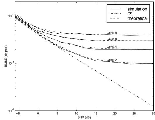
Fig. 2. Comparison of the RMSE of the DOA estimates based on simulation and theoretical values of (27).
