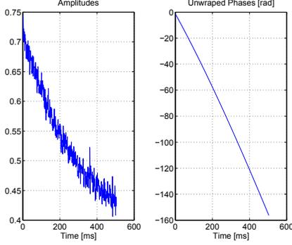
**Fig. 2.** Time Varying Amplitude due to Scattering Radiation on Rough Surface ( $\gamma = 0.25$ ).
