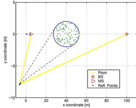
**Fig. 1.** Scattering on Rough Surface. (Single cluster  $p = 1$ , the number of reflection points  $q_1 = 100$ , the reflection points are uniformly distributed in a circular area with radius  $0.25\lambda$ , the number of channel samples  $N = 500$ , the mobile velocity is  $10m/s$ , the distance from BS to the center of gravity of the scattering surface is  $100$  m, the distance from MS to the center of gravity of the scattering surface is  $10$  m, and the SNR is  $10$  dB.)
