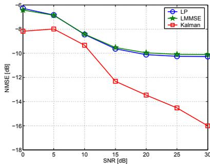
**Fig. 3.** Performance evaluation using simulated data. ( $\gamma = 0.25$ , prediction horizon  $L=5$  (around  $0.3\lambda$ ))
