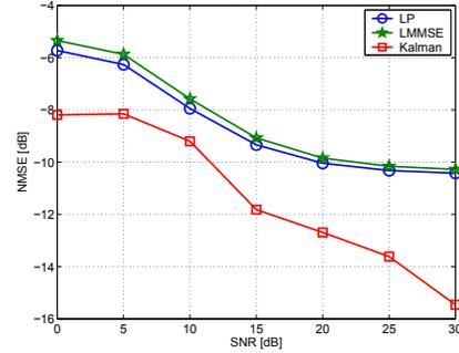
**Fig. 4.** Performance evaluation using simulated data. ( $\gamma = 0.5$ , prediction horizon  $L=5$  (around  $0.3\lambda$ ))
