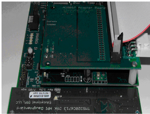
Fig. 3. Adapter board and FPGA daughtercard stacked on top of a TI C6713 DSK. The HPI daughtercard in the foreground is required to operate this system from winDSK6.
