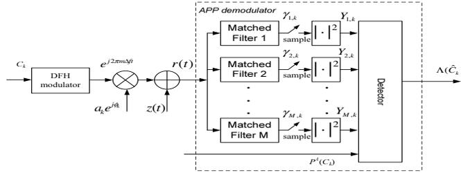
**Fig. 1.** Equivalent baseband DFH receiver with an APP demodulator.
