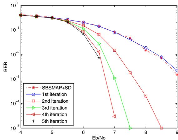
**Fig. 3.** BER performance of joint iterative demodulation and decoding of DFH signals over AWGN channel, compared with the SBS-MAP detection with soft-decision Viterbi decoding of DFH signals.
