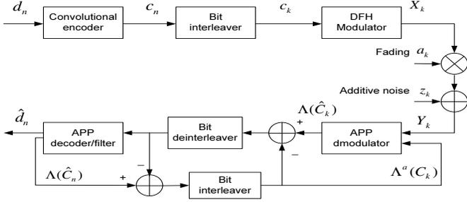
**Fig. 2.** Block diagram of the DFH system with joint iterative demodulation and decoding.
