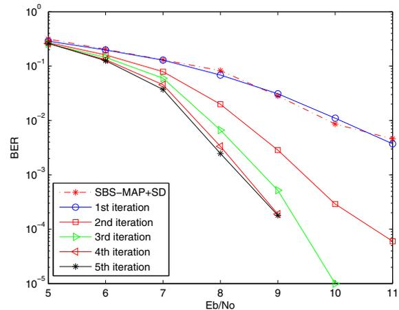
**Fig. 4.** BER performance of joint iterative demodulation and decoding of DFH signals over Rayleigh flat fading channel with fading rate  $0.05R$ , compared with the SBS-MAP detection with soft-decision Viterbi decoding of DFH signals.
