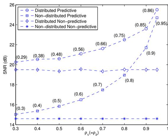
**Fig. 2.** Performance comparison of distributed predictive scalar quantizers with other alternatives at the rate of 3 bits/sample per source, 1st-order prediction, and  $\gamma = 0.98$ . The number in parenthesis is the predictor coefficient.
