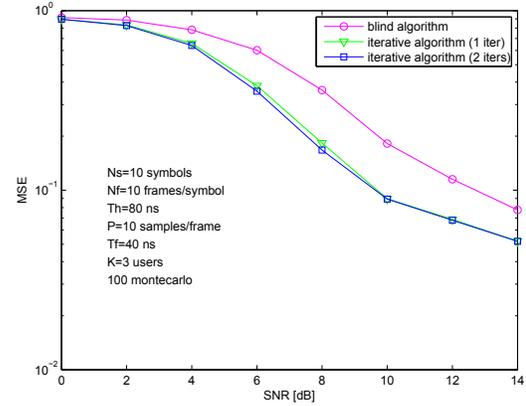
Fig. 4. Channel MSE vs. SNR performance for CM1
