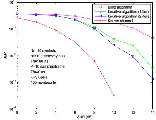
Fig. 7. BER vs. SNR performance for CM2
