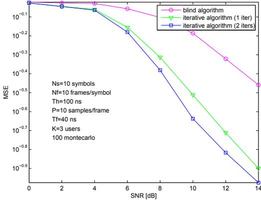
Fig. 5. Channel MSE vs. SNR performance for CM2
