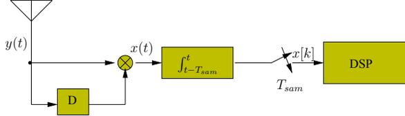
Fig. 2. Autocorrelation receiver
