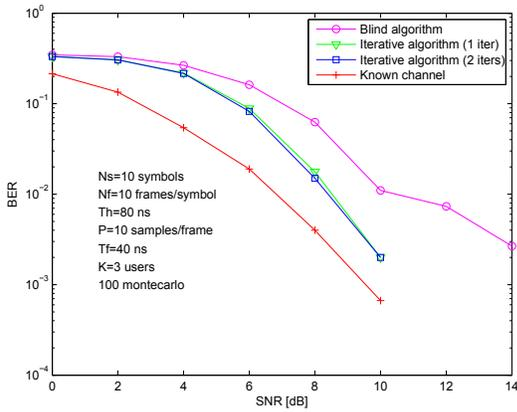
Fig. 6. BER vs. SNR performance for CM1
