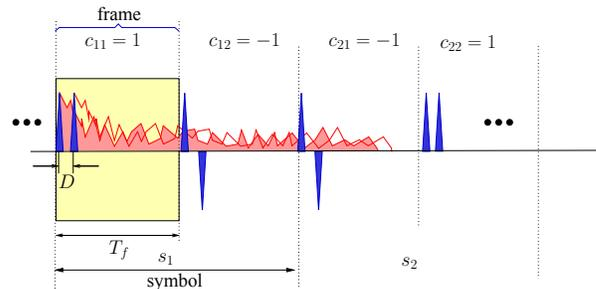
Fig. 1. Pulse sequence structure
