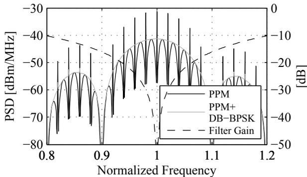
**Fig. 4: Comparison of PPM and PPM + DB-BPSK spectra (left axis), along with the filter gain (right axis).**
