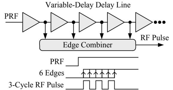
Fig. 3: Delay-line-based pulse generator architecture.
