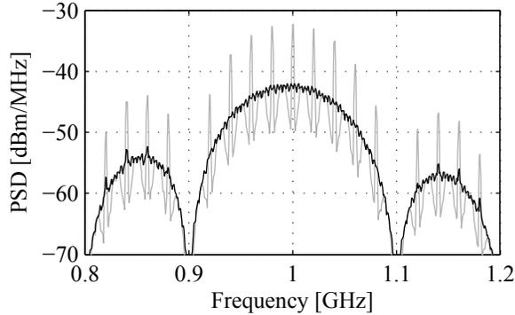
**Fig. 7: Measured spectrum for PPM (gray) and PPM + DB-BPSK pulses (black) using the AWG.**
