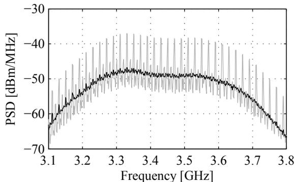
**Fig. 8: Measured spectrum for PPM (gray) and PPM + DB-BPSK pulses (black) using the custom RFIC.**
