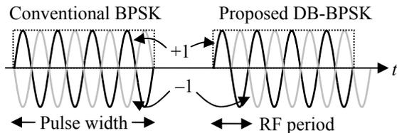
Fig. 2: Conventional and delay-based BPSK.
