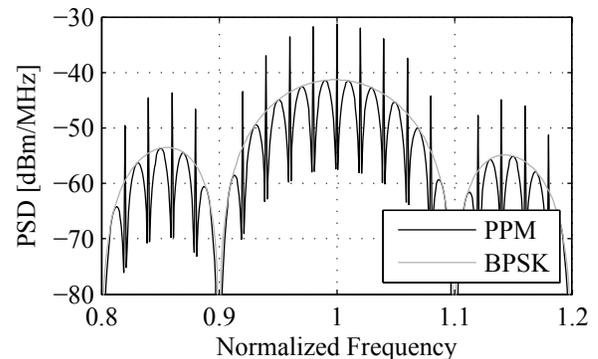
Fig. 1: Comparison of PPM and BPSK spectra with equal total pulse energy at a 10MHz PRF.
