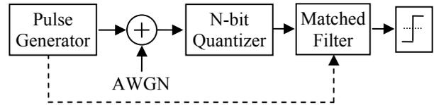
**Fig. 5: Receiver architecture implemented in Matlab for BER performance simulations.**
