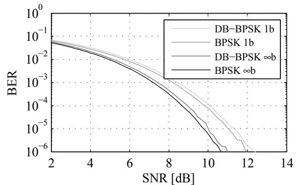
**Fig. 6: Waterfall curves of a matched-filter DB-BPSK and BPSK system with a 1 bit ADC and no ADC.**
