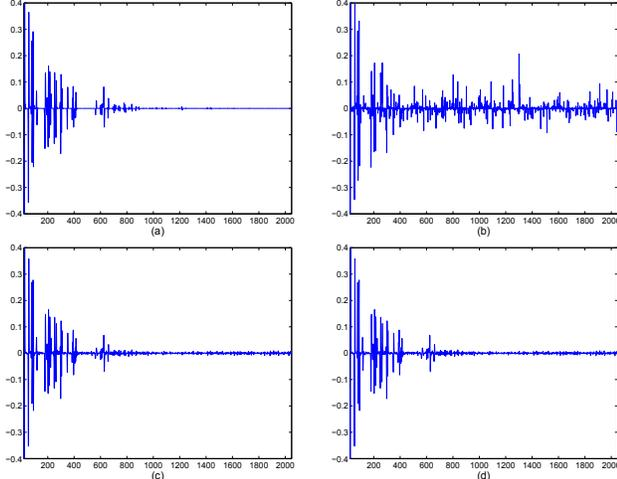
**Fig. 2.** (a) Received UWB signal; (b) CS reconstruction using time-sparsity model,  $K = 500$ . CS reconstruction using multipath diversity with: (c)  $K = 500$  and (d)  $K = 250$ .
