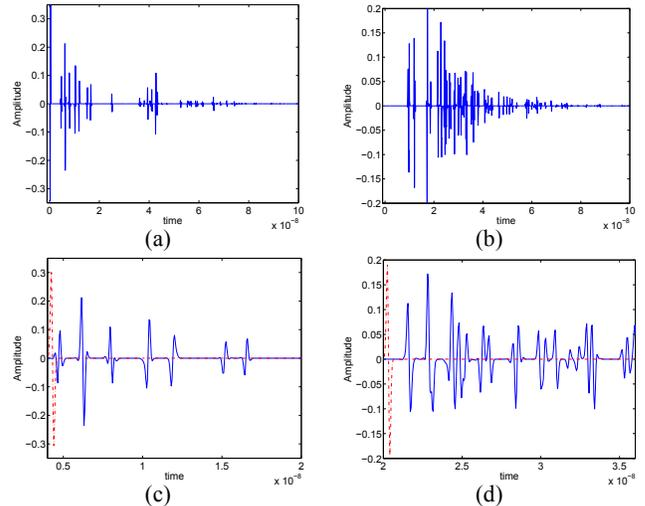
**Fig. 1.** Effect of UWB channel (indoor residential environment) on the transmitted pulse for two different propagation scenarios (a) LOS; (b) NLOS; (c) Zoom-in of (a); (d) Zoom-in of (b); Transmitted pulse (---) is also shown in (c) and (d).
