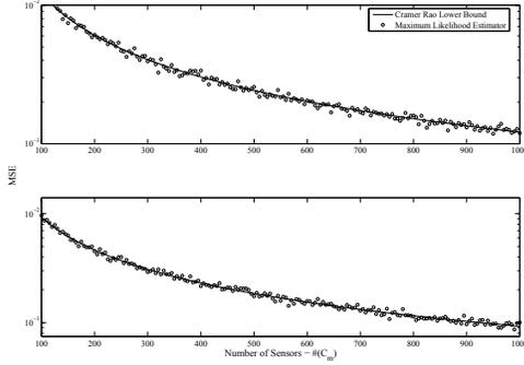
**Fig. 1.** Illustration of ML (circles) estimator output variance along with the CRLB (solid) where  $M = 3$ ,  $\sigma_1 = 1$ ,  $\sigma_2 = 2$ ,  $\sigma_3 = 1.5$ ,  $\theta = 1$  (top:)  $\tau = 0$  and (bottom:)  $\tau = 1$ .
