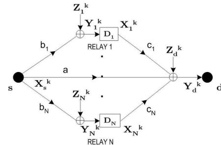
Fig. 1. Multiple relay channel with linear relaying functions.
