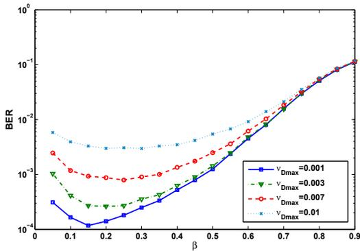
Fig. 2. Simulations-based BER versus  $\beta$  (25) for SNR=15 dB.
