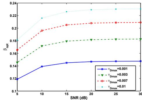
Fig. 3. Theoretical  $\beta_{\text{opt}}$  (28) versus received signal SNR
