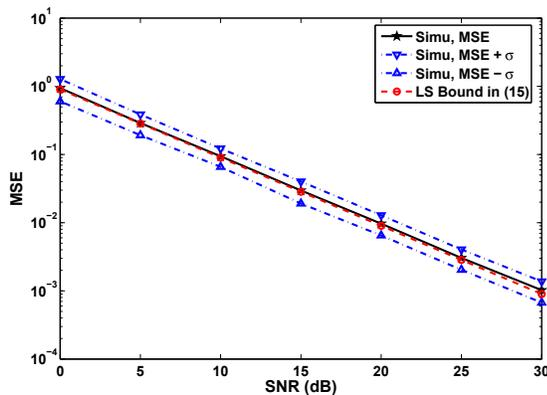
Fig. 1. Comparison between channel estimation MSE lower bound in (15) and simulation-based results.  $\nu_{D\max}=0.001$  i.e.  $f_d=40$  Hz
