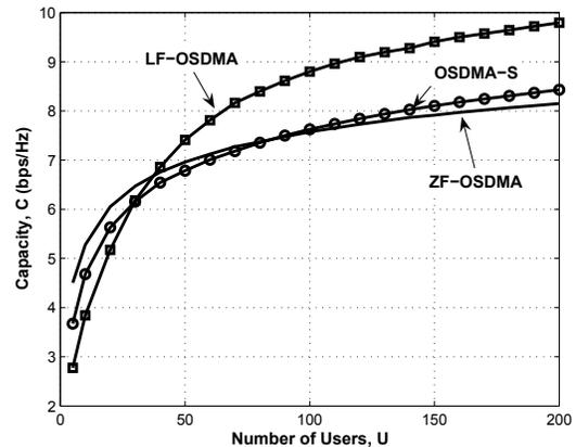
Fig. 2. Performance comparison between LF-OSDMA, ZF-OSDMA and OSDMA-S for the number of antennas  $N_t = 4$ , CSI feedback no larger than 6 bits/user and SNR = 5 dB.
