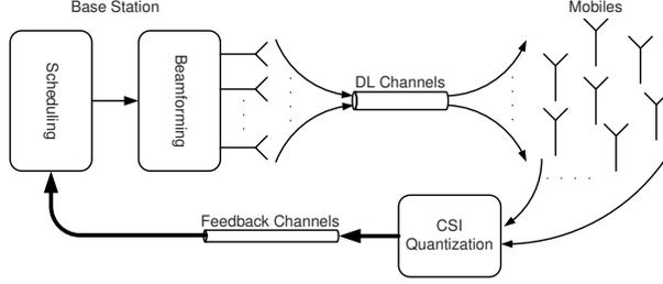
Fig. 1. Downlink system with limited feedback
