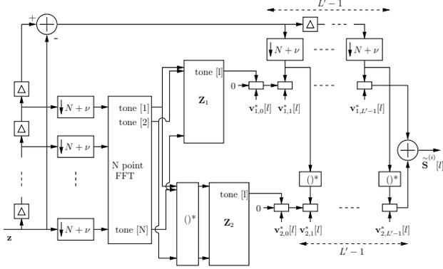
Fig. 1. PTEQ for OFDM with IQ imbalance
