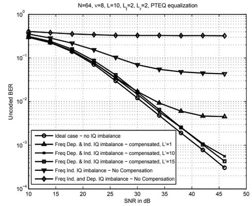
(b) 10-tap complex Gaussian channel (fading)
