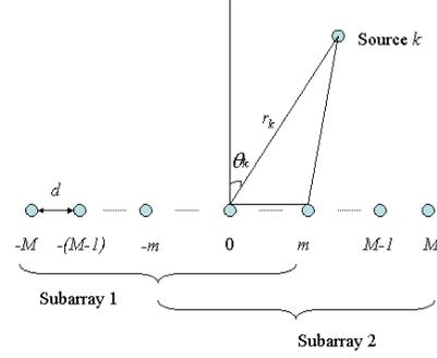
Fig. 1. Near field ULA configuration with symmetric partition.
