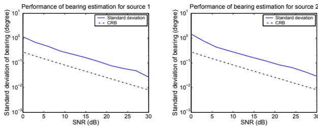
Fig. 2. Standard deviation and CRB versus SNR of the bearing estimation.
