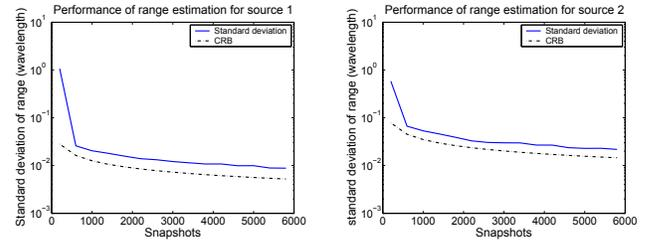
Fig. 5. Standard deviation and CRB versus snapshots of the range estimation.
