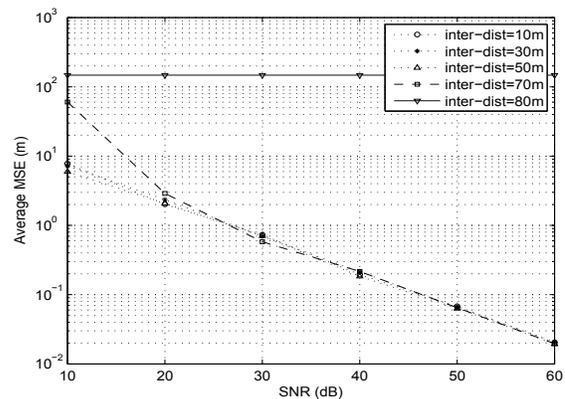
Figure 2. MSE vs SNR for various inter-sensor spacing
