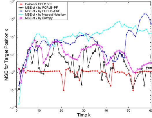
**Fig. 2.** Comparison of *posterior* CRLB to MSEs for the x-coordinate of target position calculated using different sensor selection methods.
