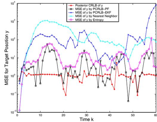
**Fig. 3.** Comparison of *posterior* CRLB to MSEs for the y-coordinate of target position calculated using different sensor selection methods.
