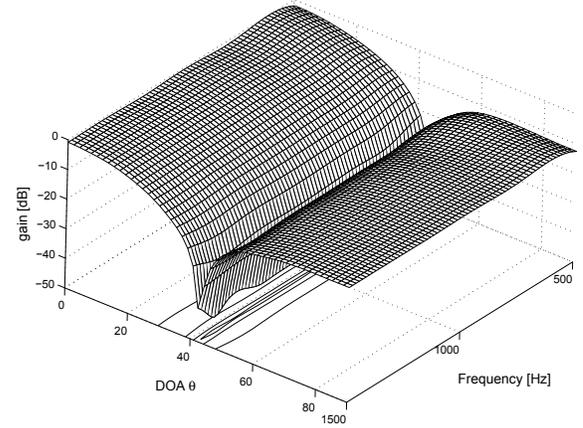
Fig. 4: A slice of the beam pattern  $(\theta, f)$  at azimuth angle  $\phi = 100^\circ$ .
