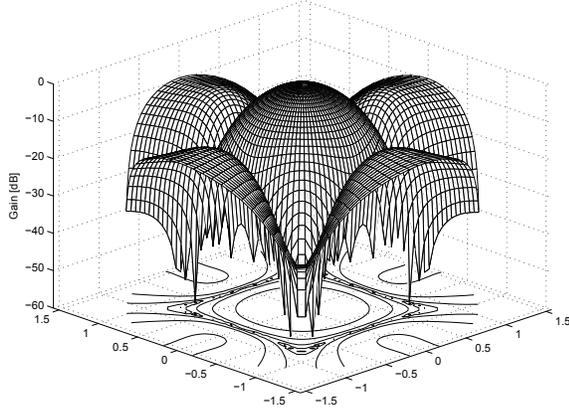
Fig. 2: The resultant beam pattern of the 3-D array at  $f = 500\text{Hz}$ , with respect to azimuth (angle coordinate) and elevation (radial coordinate).
