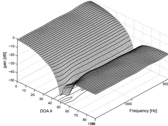
Fig. 5: A slice of the beam pattern  $(\theta, f)$  at azimuth angle  $\phi = 300^\circ$ .
