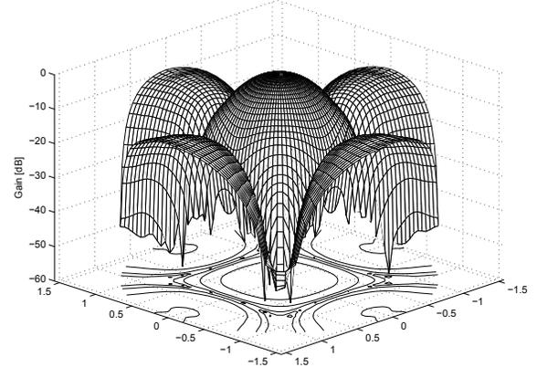
Fig. 3: The resultant beam pattern of the 3-D array at  $f = 1500\text{Hz}$ , with respect to azimuth (angle coordinate) and elevation (radial coordinate).
