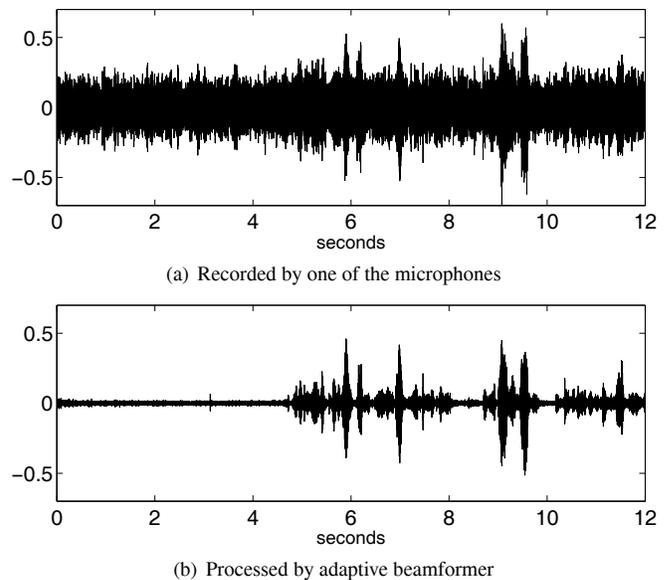
Fig. 5. Processed recorded signal with bandlimited noise interference
