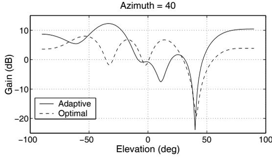
Fig. 2. Spatial response at 1.5 kHz, with the interference at azimuth  $40^\circ$  and elevation  $40^\circ$
