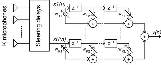
Fig. 1. Block diagram of the LCMV beamformer
