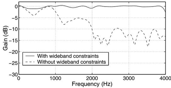
Fig. 3. Frequency response to the off-steering desired signal
