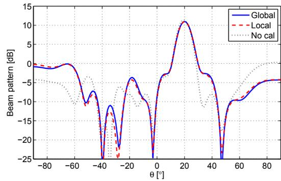
**Fig. 1.** Beam pattern using a Taylor taper (three side lobes 30 dB below main lobe maximum) and optimal SNR calibration with different correction matrices.
