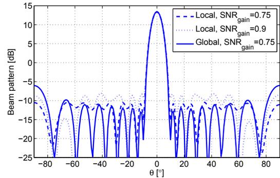
**Fig. 4.** Beam pattern from optimization. Position and channel errors.
