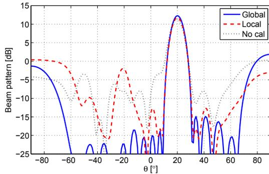
**Fig. 2.** Beam pattern using a Taylor taper (three side lobes 30 dB below main lobe maximum) and virtual array calibration with different correction matrices.
