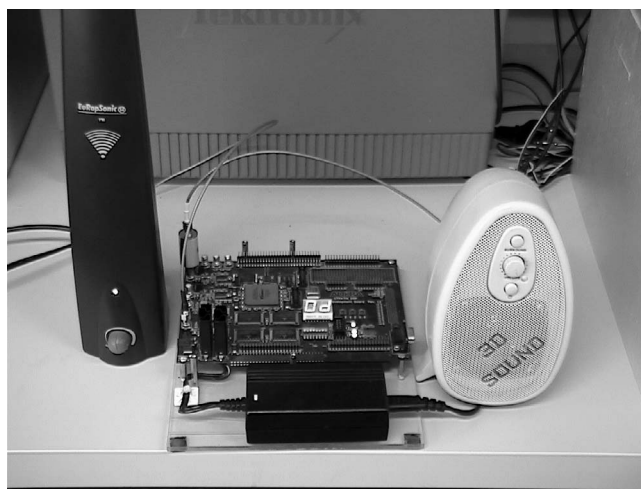
Figure 1. Photograph of the indexing engine prototype, showing RF front end, FPGA card with user interface, and loudspeaker.
