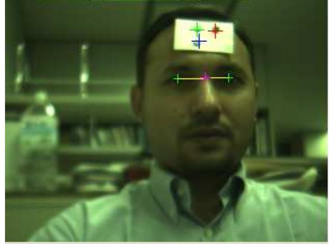
**Fig. 3.** Marker object on the forehead for the marker based pose estimation.
