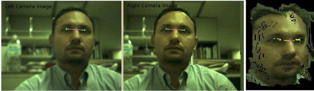
**Fig. 1.** Screen capture of the left and right camera images, and OpenGL plot of texture mapped 3D point clouds reconstructed by the stereo algorithm.
