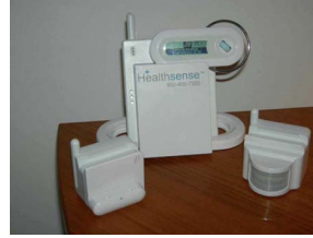
Fig.1. (a) The data acquisition platform which combines static home and wearable wireless sensors. (b) The static home sensors. (c) Wearable wireless sensor kit attached to the right wrists.
