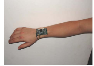
Fig.1. (a) The data acquisition platform which combines static home and wearable wireless sensors. (b) The static home sensors. (c) Wearable wireless sensor kit attached to the right wrists.
