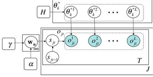
**Fig. 2.** The infinite hidden Markov model interpreted as an HDP. For observation  $o_{jt}$ ,  $s_{jt-1}$  defines the mixture model to be used and  $s_{jt}$  selects the mixture component according to infinite dimension weight vector  $w_{s_{jt-1}}$ .
