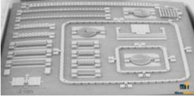
Fig. 1. Microfabricated MEMS Test Structures.
