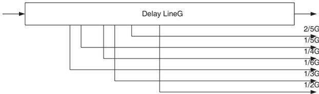
Fig. 4. Shared Farey fraction delays
