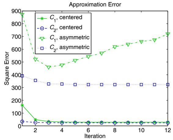
**Fig. 3.** Convergence of approximation error. The word ‘centered’ refers to the desired beampattern in Fig. 1 and ‘asymmetric’ to that in Fig. 2. Using  $C_2$  results in faster convergence and lower squared error.
