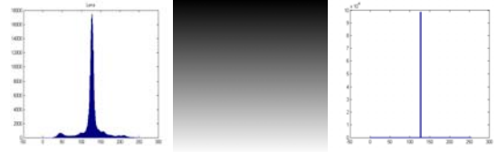
Fig. 5 (Left) Histogram of coefficients of Lena image (Mid) Artificial image with exactly flat histogram (Right) Histogram of the coefficients of the artificial image
