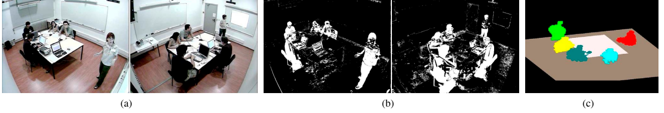
Fig. 1. In (a), a sample of multiview original images. In (b), foreground segmentation of the input images employed by the SfS algorithm. In (c), example of the binary 3D voxel reconstruction used in this paper (false colors are employed to depict various people).
