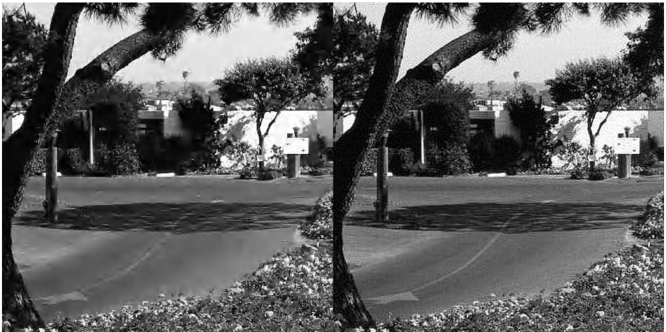
Fig. 3. “Rose” image compressed to 0.5 bits per pixel with JPEG2000 (left) and PIC 8x8 (right). The JPEG2000 image has PSNR=23.2 and WCWSSIM=0.88 while the PIC 8x8 image has PSNR=21.6 and WCWSSIM=0.94.
