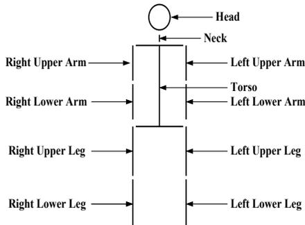
Fig. 1. Kinematic linked structure
