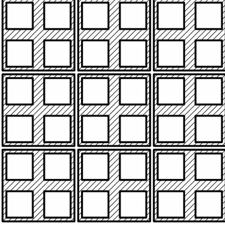
**Fig. 1.** Array structure of photodetectors: small squares represent the photodetectors for HR image and hatched squares represent the ones for LR image
