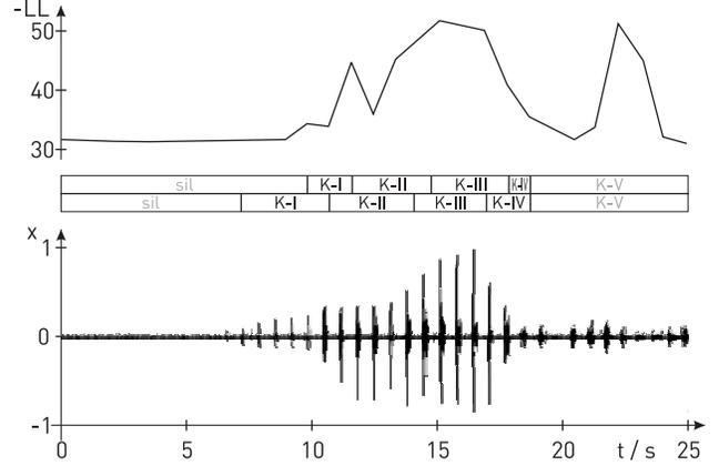
**Fig. 4.** Automatic labeling of a Korotkoff sound (bottom of figure). The second channel from the bottom shows the labeling result, the third channel the manually set reference labels. The upper channel shows the neg. log-likelihood scores computed for the respective signal segments.
