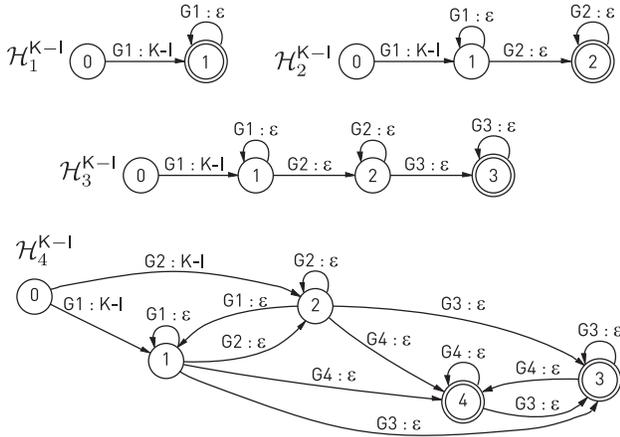
**Fig. 3.** Tested HMM topologies  $\mathcal{H}_1 \dots \mathcal{H}_4$ .  $G_n$  denote Gaussians associated with the transitions.
