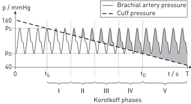
**Fig. 2.** Brachial artery and cuff pressure over time during a blood pressure measurement.
