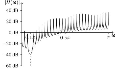
Figure 6: Magnitude responses of prediction error filters when used to predict a single sinusoid at  $\omega = 0.1\pi$  for an all-pole filter (solid line) and a zero-only filter (dotted line).
