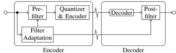
Figure 1: Overview of previous ultra-low-delay audio coding systems by Schuller *et al.*
