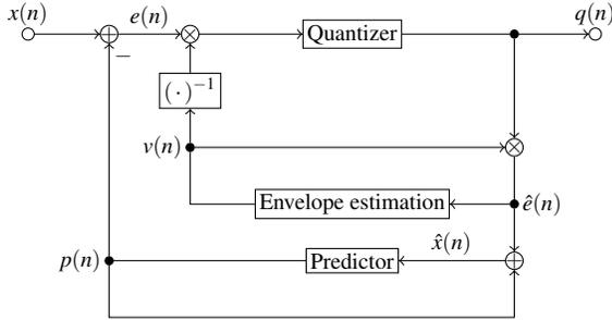
Figure 3: Structure of the ADPCM encoder.
