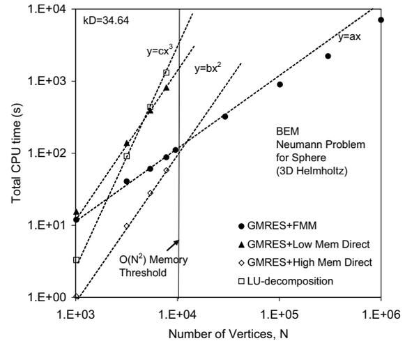
**Fig. 2.** The performance of the various components of our FMM BEM software on a test problem at various sizes. For comparison the performance of a typical BEM direct software package, and a BEM iterative package are also shown.
