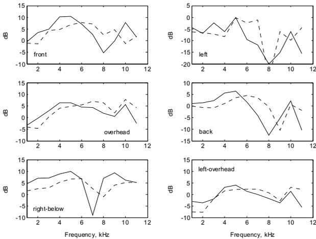
**Fig. 4.** Comparison of computed and measured HRTFs in the CIPIC database [1] for selected positions.
